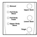
Thigh buttons. Pressing a button once will activate a massage zone. Pressing the button again will turn off the massage zone. Press the buttons to activate the desired massage zones.
